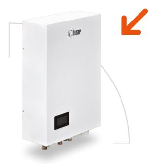
The **SMART** unit contains a controller offering many functions for the user, an electronic installation manual, a supplementary electric heater, a central heating/hot tap water switch valve, and a circulation pump. It is connected with the external unit by means of a communication cable included with the device.
