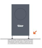
Height-adjustable feet for installation on solid substrate
